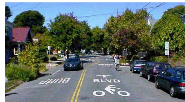
On bike boulevards, the road is marked to encourage bicycling, but bikes are not directed into separate lanes from motor vehicle traffic.
