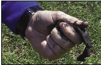
Ribbon test used to estimate clay content.
