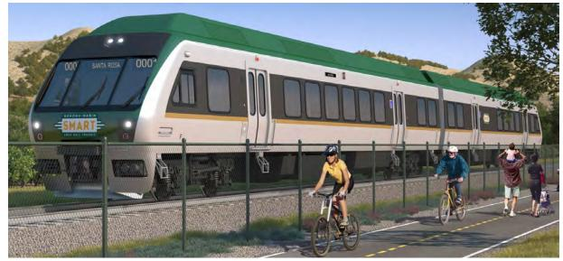
Figure 12: Typical Two-Car Trainset of New FRA Compliant DMU Equipment
