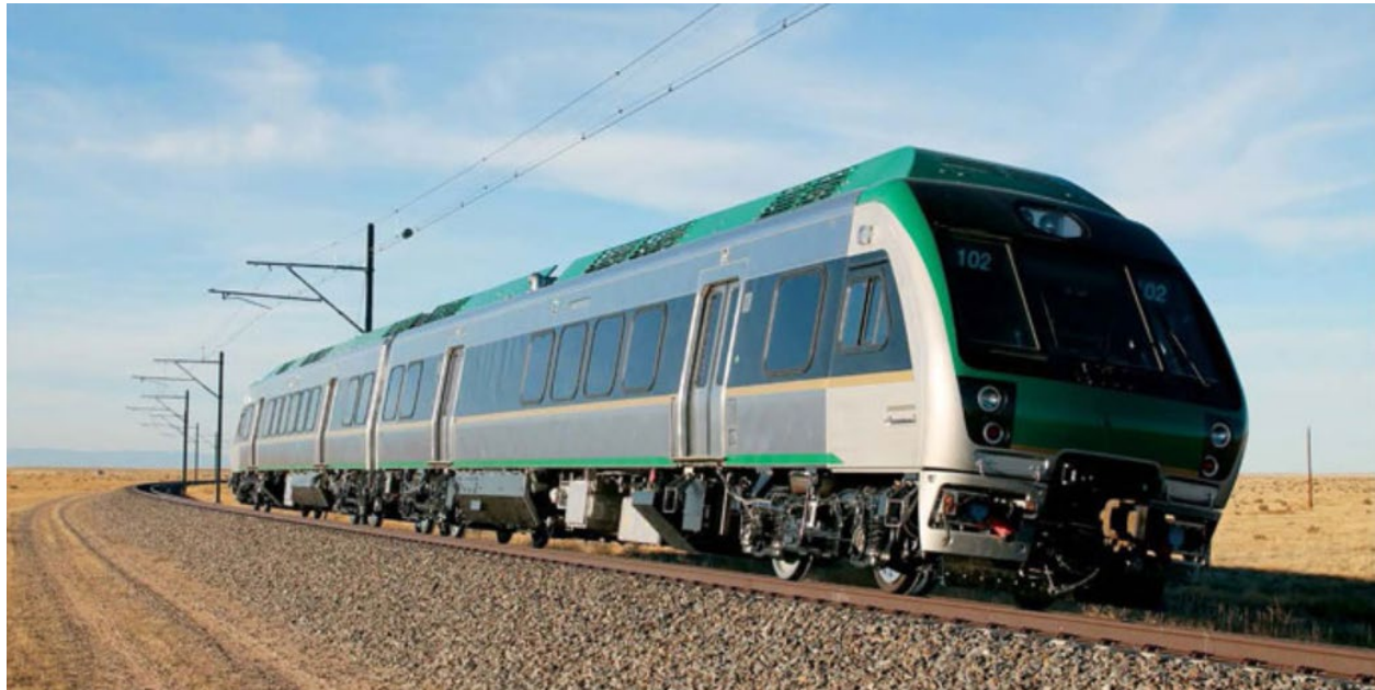
Figure 16: Typical Two-Car Trainset of New FRA Compliant DMU Equipment
