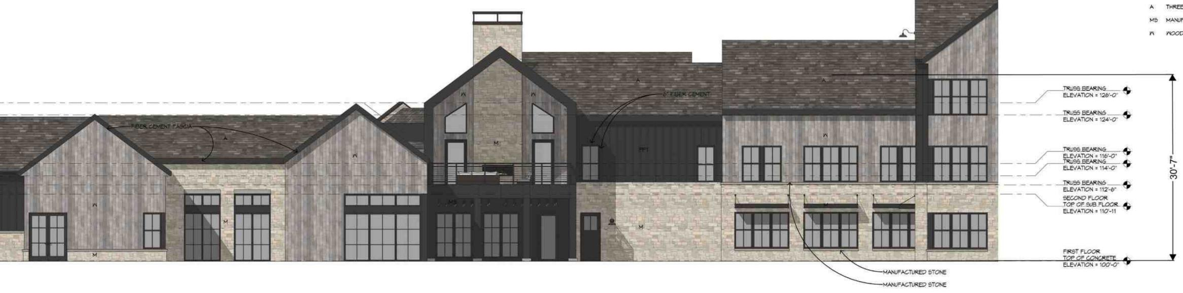
2. ALL CONDUIT, METERS, VENTS, ETC. TO BE PAINTED TO MATCH ADJACENT SURFACE. 3. GUTTERS AND DOWNSPOUTS ARE PREFINISHED ALUMINUM.
