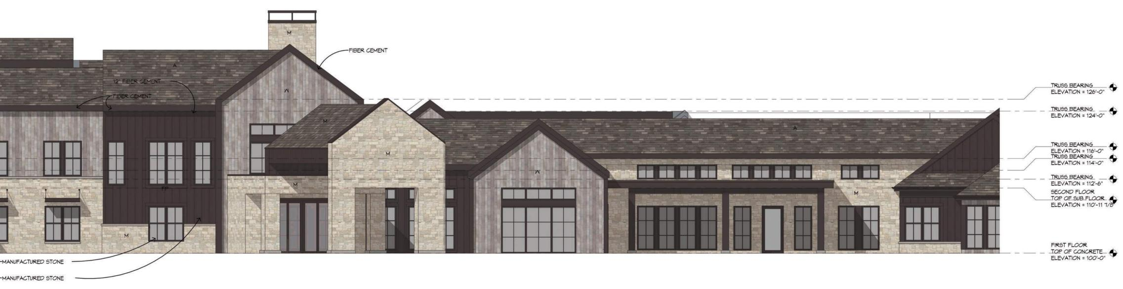
2. ALL CONDUIT, METERS, VENTS, ETC. TO BE PAINTED TO MATCH ADJACENT SURFACE. 3. GUTTERS AND DOWNSPOUTS ARE PREFINISHED ALUMINUM.
